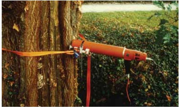
Figure 2. First portable resistance drill series (1987), based on the results of a physics master thesis, built by the German company Fein, and sold to experts worldwide. Görlacher and Hättich (1990) proved a linear correlation of its profiles to wood density.
