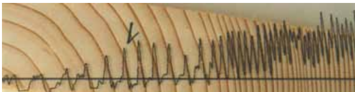
Figure 7. Broad conifer rings are usually dominated by soft earlywood. Due to age trend (Bräker et.al. 1981) in ring width, conifers (trees, beams, and poles) are mostly much softer in the center. The corresponding decline in drill resistance can only be distinguished from a decline by internal decay if the intra-annual density structures are revealed correctly. This requires a high-resolution profile, measured and recorded electronically; other profiles will lead to mis-interpretation and wrong evaluation of trees and timber.
