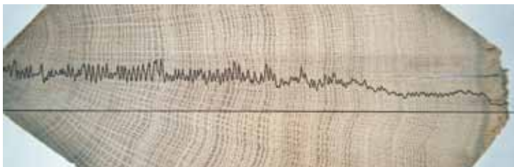
Figure 8. Broad, ring-porous tree rings are dominated by dense latewood. Due to age trend in ring width, ring-porous trees, branches, or beams are denser in the center, leading to an increasing drill resistance. Narrow oak ( Quercus ) rings are dominated by soft earlywood, leading to a drop in density and drill resistance profiles. High-resolution electronic drills are mandatory for distinguishing such zones of narrow but intact rings from areas of decay, where the profile drops down below earlywood level.
