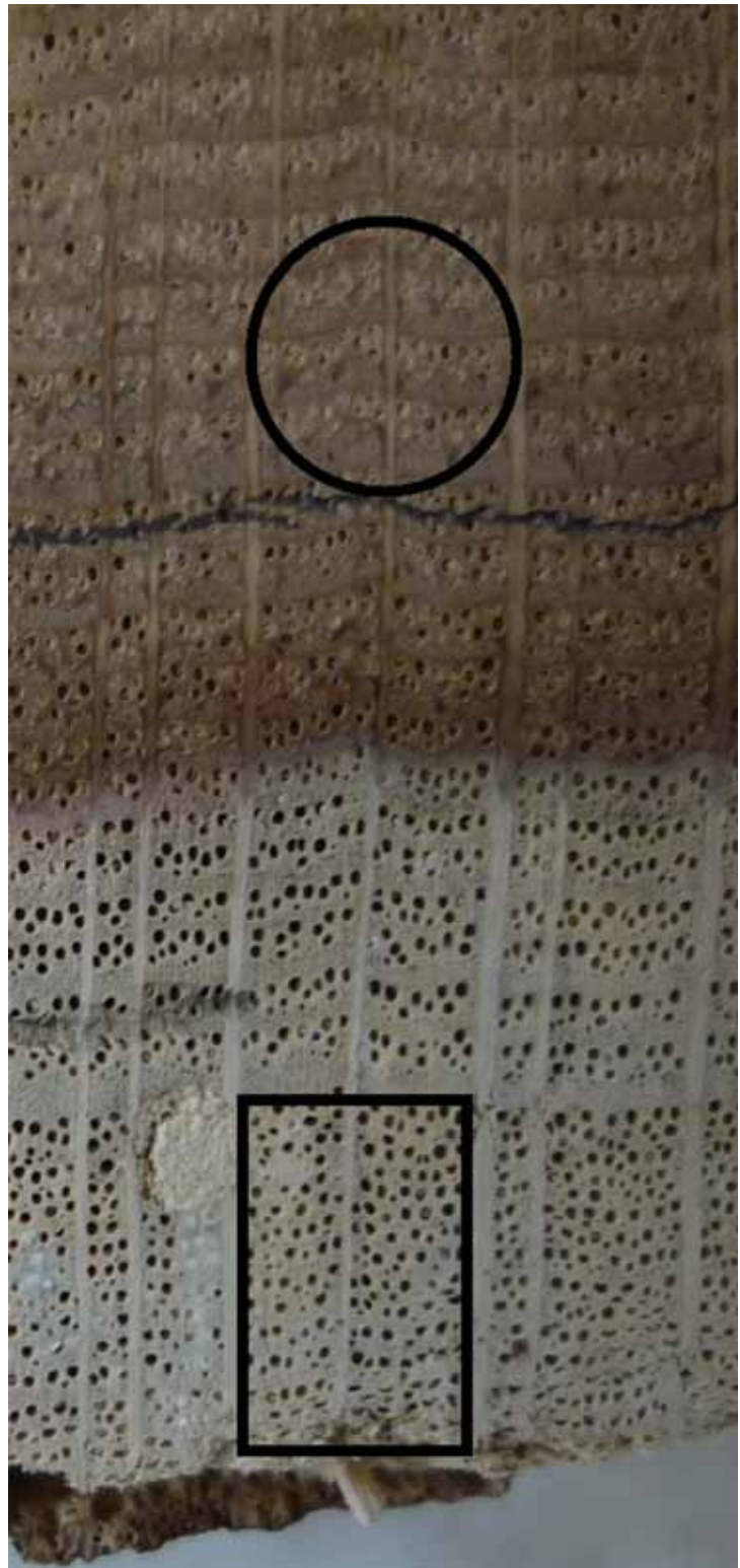
Figure 6. Typical example of declining oak tree-ring width with age. In the center of such stems, big latewood zones are visible (circle), leading to a high density. Closer to the bark, the narrowing rings may only consist of big earlywood vessels for water transport (rectangle). As a result, local wood density is very low, even lower than common in softwood species. Thus, the slower a ring-porous tree grows, the higher the relative amount of earlywood in the tree rings and the lower the density of the wood. However, this effect is not correlated to durability of the wood as this is mainly determined by the content of resin/tannins and other impregnating substances.
