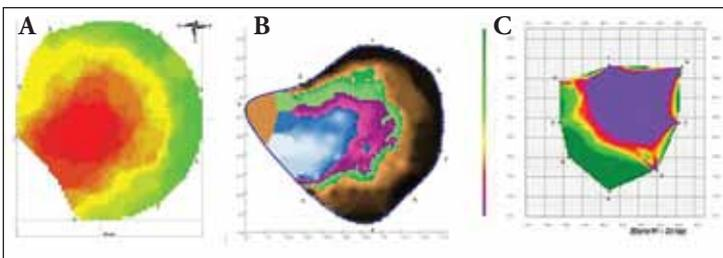
Figure 3. Device results: a) ARBOTOM, b) PICUS, c) FAKOPP 2D.
